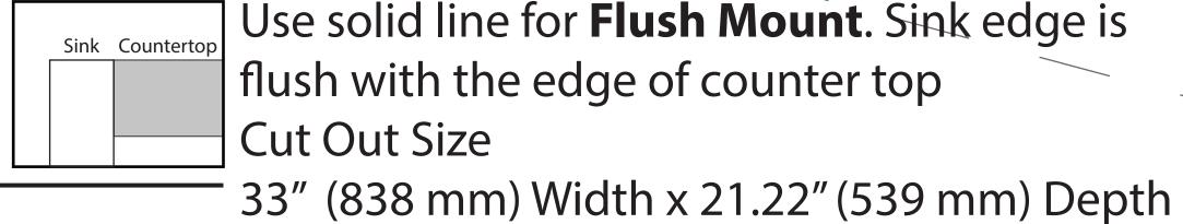
Use solid line for Flush Mount. Sink edge is flush with the edge of counter top Cut Out Size
