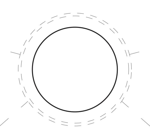
Use dotted line for **Under Mount**. Sink rim is about 1/2" (12.5 mm) revealed from the edge of the counter top opening. Cut Out Size
